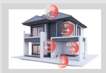
Building's envelope, especially walls, contributes to as much as 45% of the energy required in buildings. Good thermal insulation for the envelope is crucial to prevent heat from seeping in through the exterior of the building. In the Middle East particularly when a lot of energy is consumed for cooling of buildings, the use of good insulation can be very beneficial as it keeps cool air sealed within the buildings.
